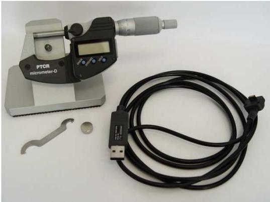
2. Unscrew the battery cover at the backside of the micrometer, remove the battery packaging and insert it with the positive terminal outward. After that properly mount the battery cover.
